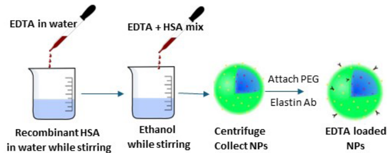
Figure S1 Formulation of anti-elastin antibody coupled EDTA-loaded albumin nanoparticles. EDTA, ethylene diamine tetraacetic acid; HSA, human serum albumin; NPs, nanoparticles; PEG, polyethylene glycol; Ab, antibody.
