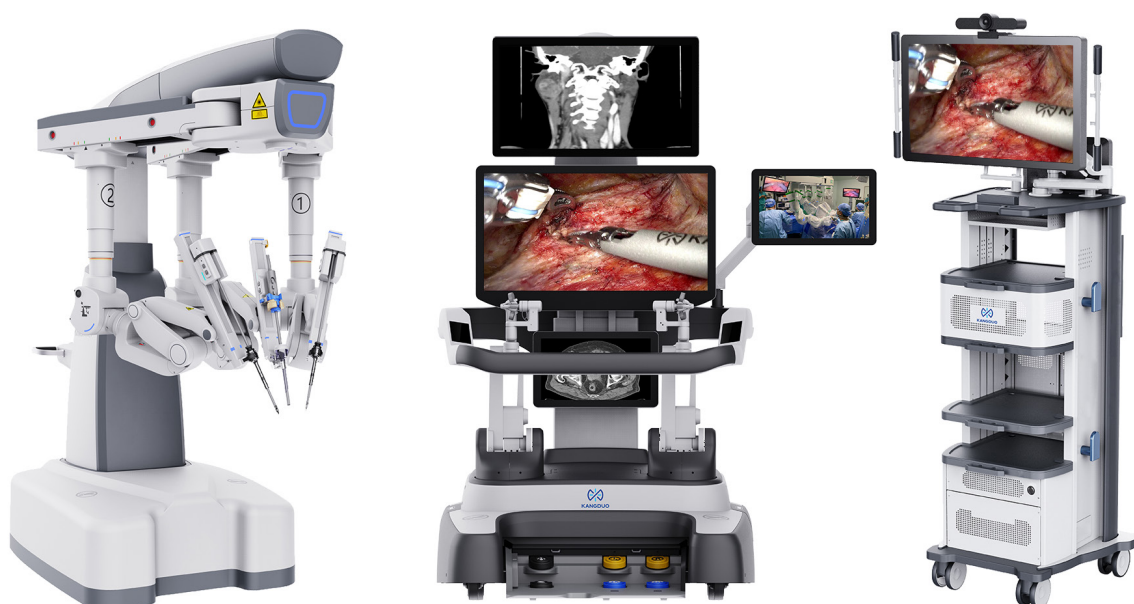
Figure 1 KD-SR-1500 system. This surgical robot consists of a patient cart (left), a surgeon control console (middle), and a vision cart (right). The figure is published with permission granted by Harbin Sagebot Intelligent Medical Equipment Co., Ltd.
